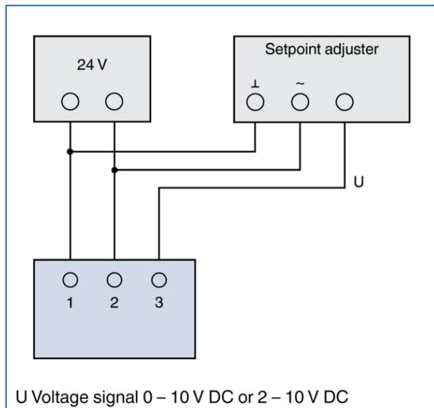
Actuators for volume flow controllers Type RN or EN
